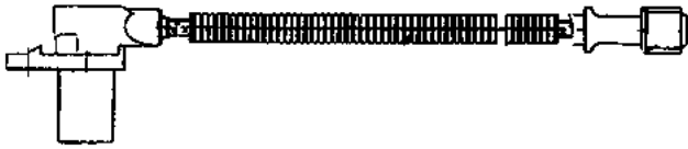
RPM SENSOR AND CONNECTION CABLE
